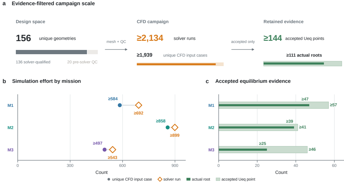
Supplementary Figure S2: Initial screening dataset. a , The dataset comprises 156 geometries, at least 1,939 unique CFD cases and at least 2,134 solver executions. Of these geometries, 136 reached the solver and 20 did not meet presolver quality criteria. At least 144 points provided equilibrium evidence, including at least 111 directly evaluated roots under the dataset definitions. Repeated or restarted calculations increase solver executions but not unique-case counts. b , CFD cases and solver executions by Mission. c , Qualified equilibrium evidence and directly evaluated roots. Counts are lower bounds for the initial screening dataset, rather than the combined total of all detailed design studies.
