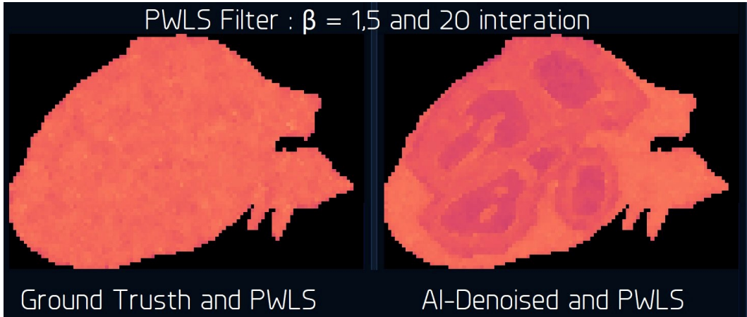
Figure 7. PWLS filter ( \beta = 1.5 , 20 iterations) applied to the Ground Truth (left) and to the Héméra image (right). PWLS erases fine gradients on the Ground Truth (characteristic over-smoothing); applied to the Héméra image, it enhances structures without degrading contrast.
